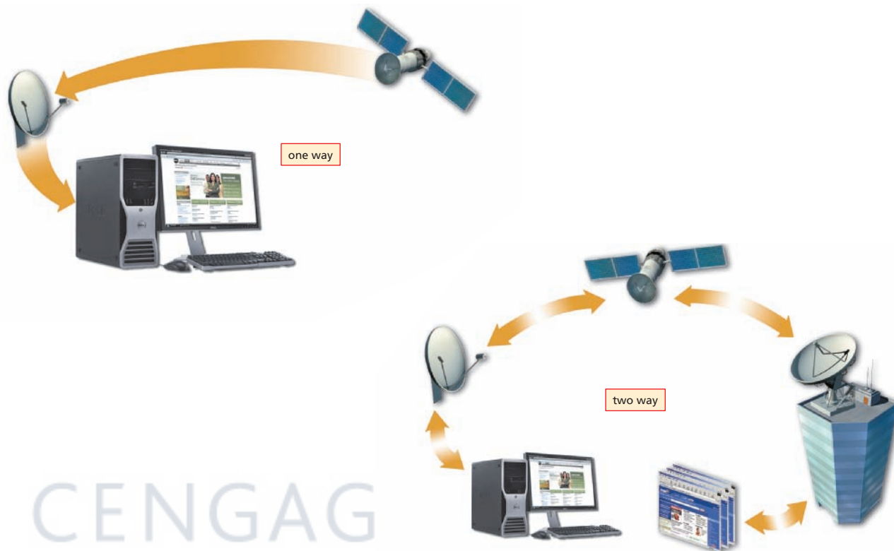
Figure 1-20 Satellite Internet access can be one-way or two-way.
