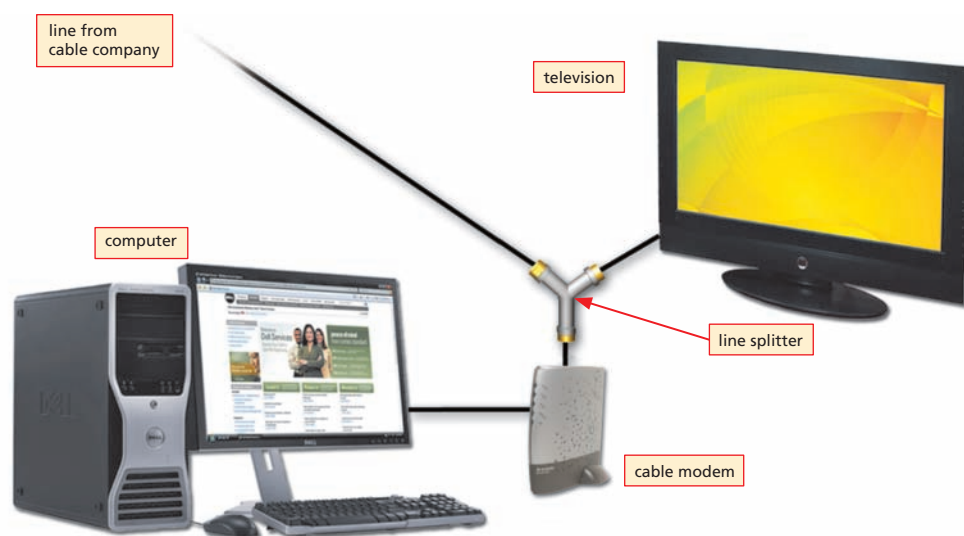
Figure 1-18 Cable Internet access requires a line splitter and cable modem.
