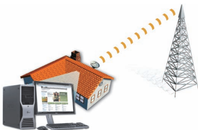
Figure 1-19 Microwave Internet access must be within line of sight to prevent signal interference.
